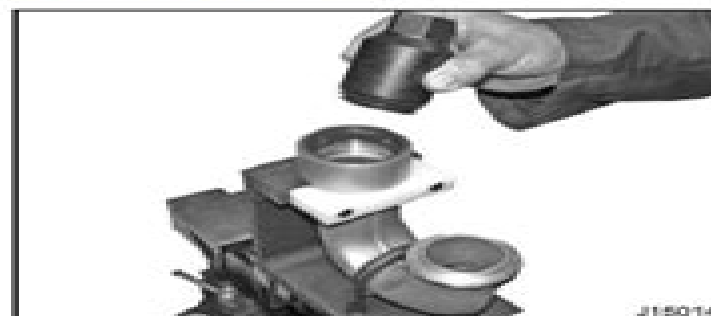
Figure 81 Installing the crossover tube seal removal tool
